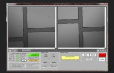
Example - adhesive bonding: Force and temperature can be adjusted in real time to improve the adhesive flow and achieve void-free bonding.
