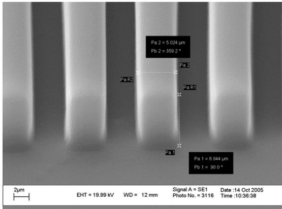
Fig 5. Vertical wall structures in PDMS on silicon
