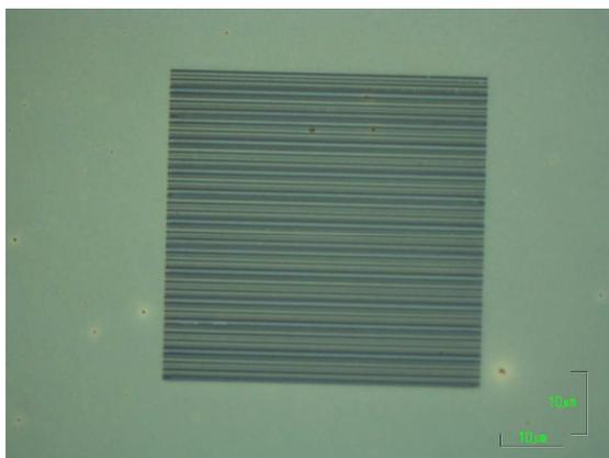
Fig 7. 100nm printed lines in surface layer
