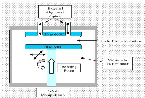
Fig 2. Schematic of process chamber
