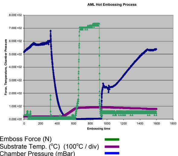
Fig 4. Data for a typical emboss process
