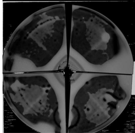
Figure 2: SAM image of wafer pair that only received wet cleaning
