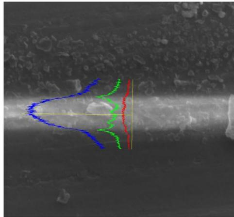
Figure 4: SEM image of bond interface for formic acid treated wafer pair
