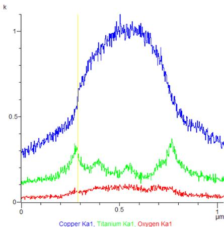
Figure 3: EDX spectra of bond interface for formic acid treated wafer pair
