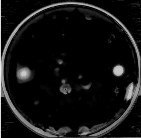
Figure 1: SAM image of formic acid treated wafer pair
